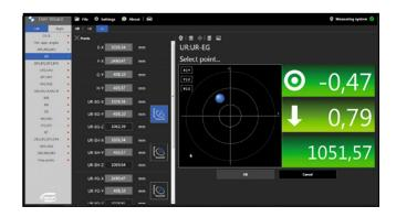
A new feature of the FMH Wizard is the crosshair, which makes it even easier to markup the points. Acoustic and visual signal indicate the distance to target in real time and help the user to move to the exact point along the interior surface.
